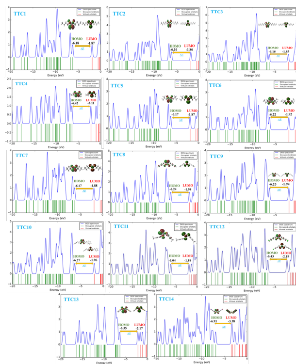
Figure 6. Calculated DOS plots of substituted trithiocarbonates ( TTC1-TTC14 ).
